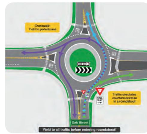
This example shows the traffic movement patterns through a one-lane roundabout. The one-lane roundabout is known as one of the safest and most efficient intersections.
